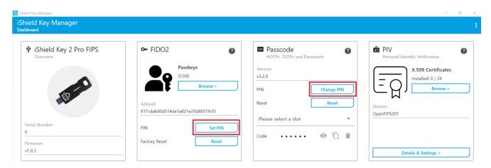
There are different "applets" depending on the iShield Key model – FIDO2, Passcode and PIV. The FIDO2, Passcode and PIV applets must be set up before they are used for the first time. To do this, open the iKM (iShield Key Manager) on the computer and set the personal PINs for each applet. These PINs must be entered for each authentication, which is done by an automatic query from the computer.
